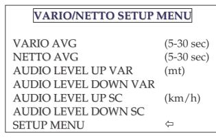
**VARIO AVG/NETTO AVG**: is the time in seconds used to calculate the average value of the VARIO and NETTO mode, with arrow  $\Rightarrow$  you can move over the avg value and change it pressing arrows  $\hat{T}$  and  $\hat{V}$ .
