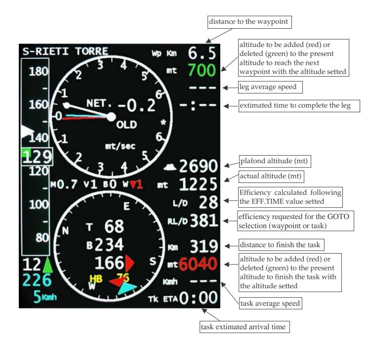
With  $\Leftrightarrow$  and  $\Rightarrow$  you can select the option McCready, Volume (is the VARIO or the NETTO volume if in the variometer on the screen you have VAR or NET), Ballast and Manual Wind. With the arrows  $\hat{T}$  and  $\hat{V}$  you can modify the selected values.
